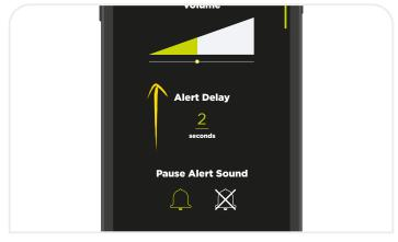
**5.** Adjust the Alert Delay to 4 seconds. This means if the connection between the Tag and the Guardian is broken for longer than 4 seconds the alarm will sound.
