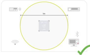
**3.** You should always try to install your Guardian at least 0.5 meters from any equipment transmitting radio signals including VHF Radios, antennas and cables.
