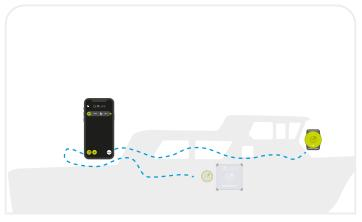
**15.** Walk around your vessel with the tag, listening out for the alarm to sound from the Guardian or the mobile device.
