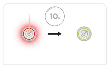
**9.** Press the control switch once. Wait 10 seconds and the system will be operating again. Solid green on the control switch indicates it is tracking correctly.
