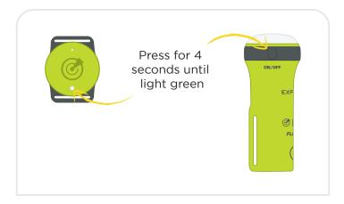
7. Switch the OLAS transmitter back ON.
