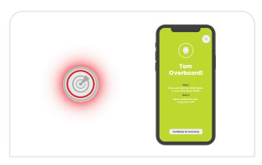
**4.** The alarm will occur after your set 'Alert Time' and the engine will cut out. The default Alert Time is 2 seconds.
