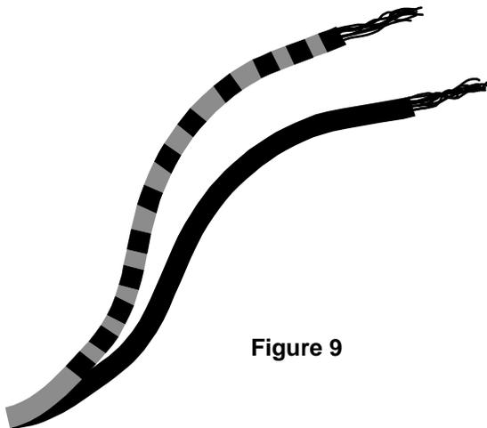
Your RapidFix™ comes with a GPS Optical Interface (transmitter plug with lead wires) and a keyed GPS bezel. The transmitter plug attaches to your RapidFix™, via the keyed bezel. The GPS Optical Interface lead wires attach to your GPS via the NMEA 0183 connector from your GPS receiver. The black lead wire with gray stripes should be connected to the **positive** transmitter pin. The black wire should be connected to the **negative** pin.
